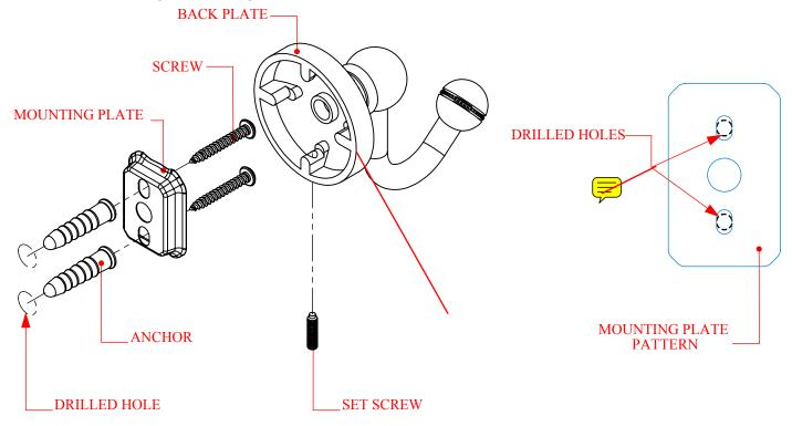
Step 2: Attach Bracket to Mounting Plate
